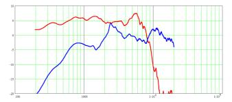
The tweeter as measured on a large baffle looks quite fine, so the problem is not in the tweeter itself. Off-axis measurements may show what the causes are.
