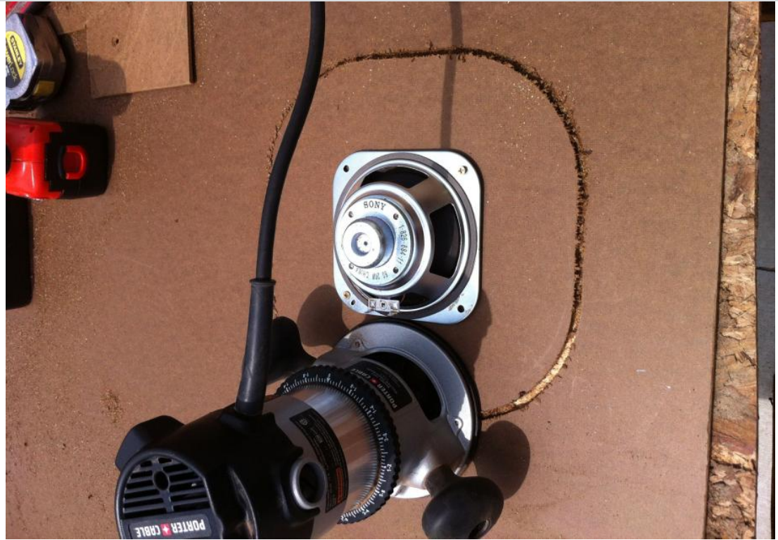
Step Six: Place new larger router base on router and use template you just made to make cutout for driver.
