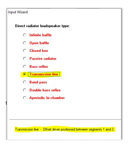
We are going to model a Mass Loaded Transmission Line (Like a long bass reflex box with a port)
