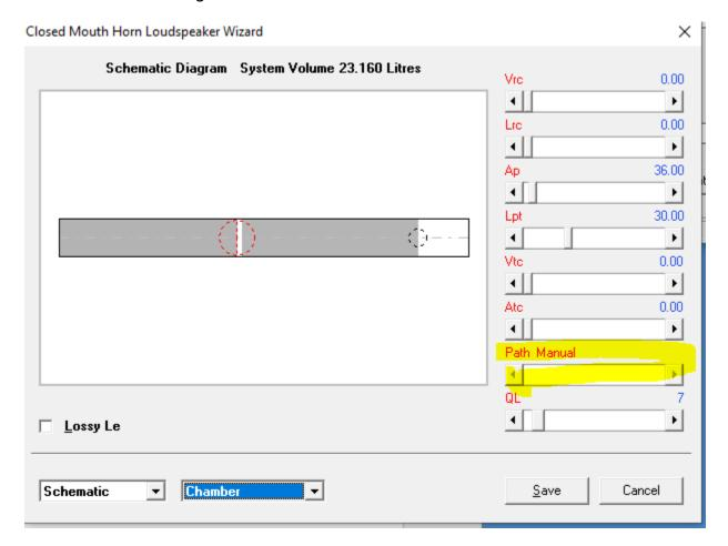
So for this design of a slim tower, with a woofer about 100 cm from the floor, and a port on the back about 18 cm from the floor and a cab that is about 38 cm front to back, the "Path" will be about 120 cm.
