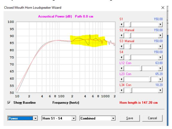
Last tip on this model, in Hornresp, "Path" is the length between the port and the driver.
