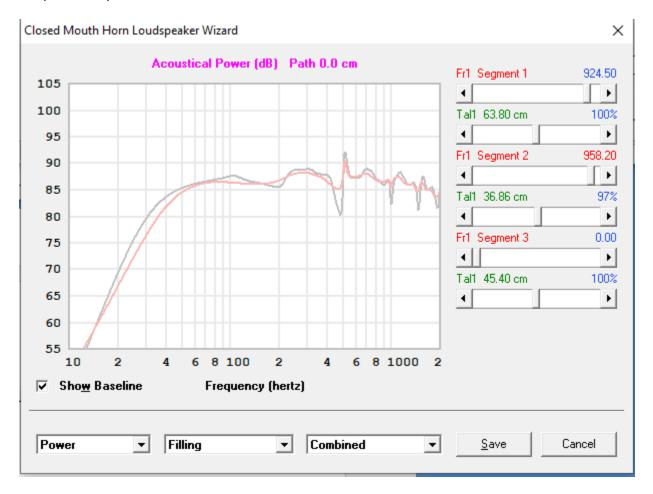
You can move the port, so I did. The distance between the center of the driver and the center of the port is L23 Con – I increased it a lot which moved the port down closer to the floor.
