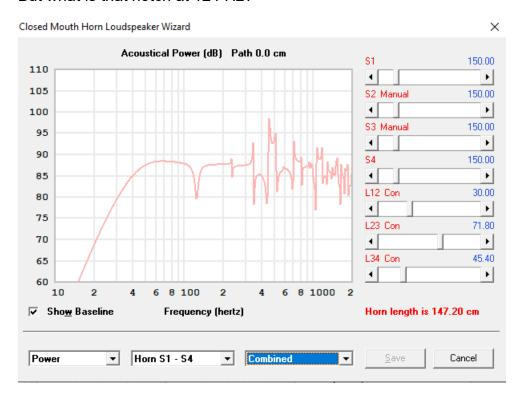
It's undoubtedly a harmonic cancellation, but we can fix it by moving the driver a bit down or up in relation to the rest of the line. So, L12 Con was at 30cm (about 12 inches).
