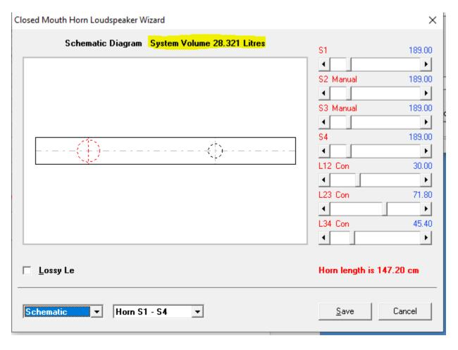
After playing with the CSA (Cross Section Area) and line lengths, we are now looking closer to the WinISD bass reflex model. F3 about 35Hz.
