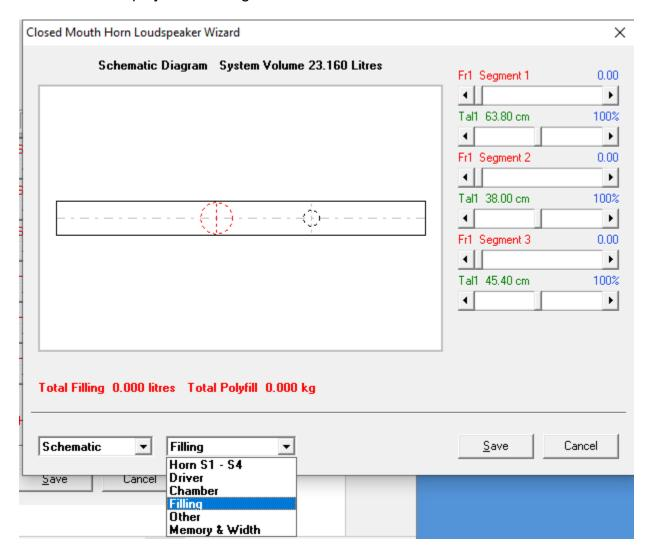
A good "Rule of Fum" is to use about "500" for stuffing and fill 100% of S1 and about 20% of S2. The Schematic view will show this to you:
