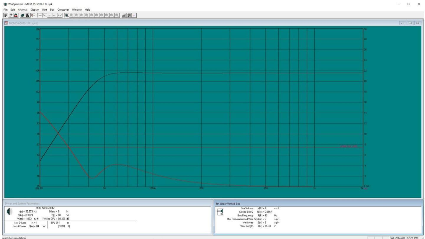
Box design with port specifications. 2" x 4.5" port was substituted to ease construction.
