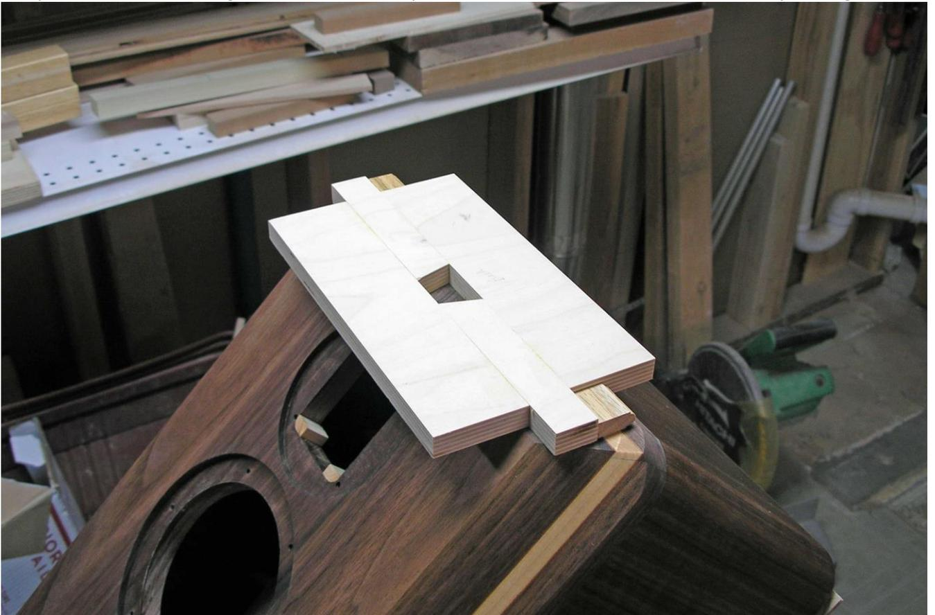
Inlay workbench setup used to cut inlay pocket with top bearing router bit.
