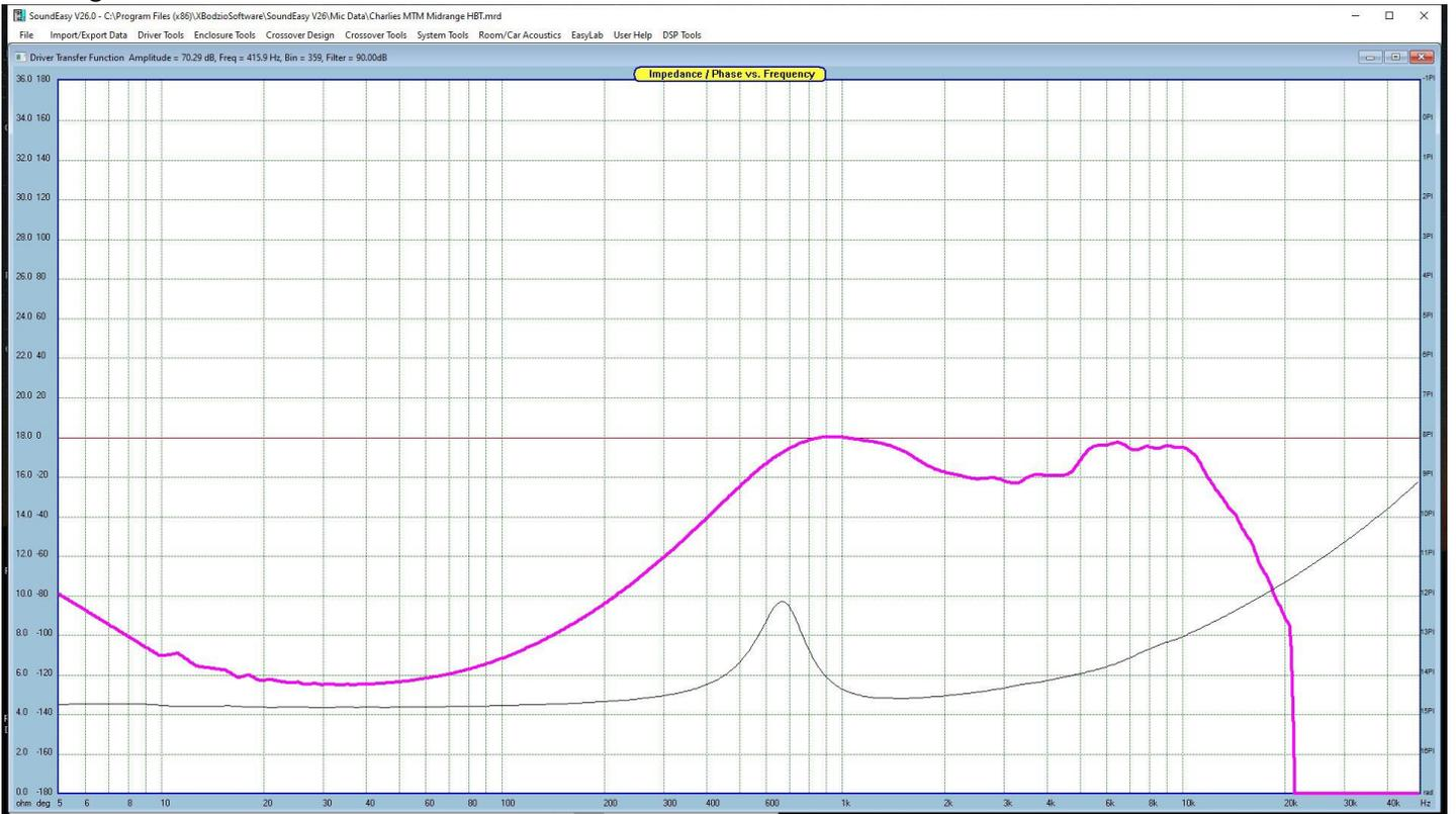
Woofer 1M far field, merged at 350Hz with NF woofer, port and calculated baffle step.
