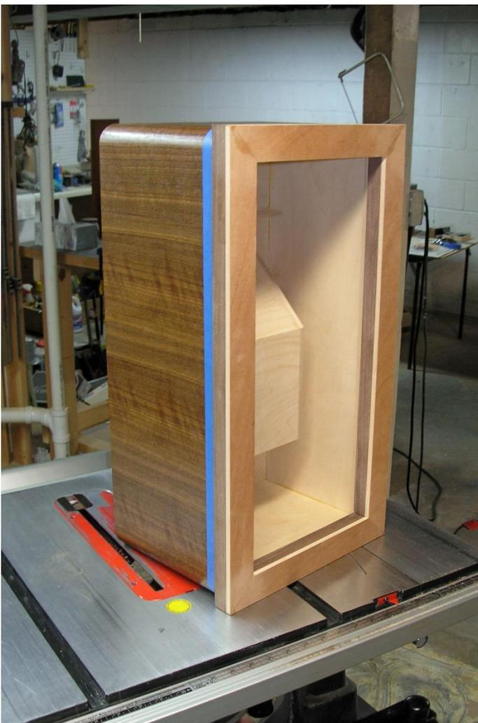
Picture frame trimmed with flush trim router bit.
