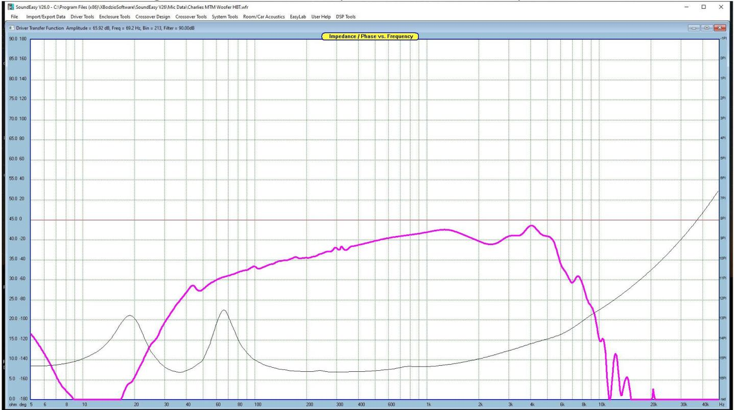
Midrange and tweeter 5Khz 24db/oct acoustic slope passive crossover.
