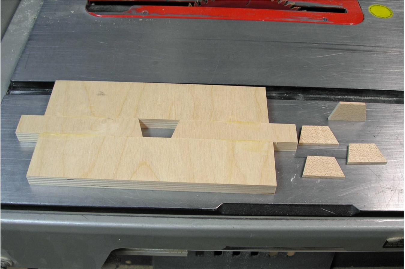
Template stuck to baffle edge with double stick tape. Note the small blocks of wood to aid template registration.
