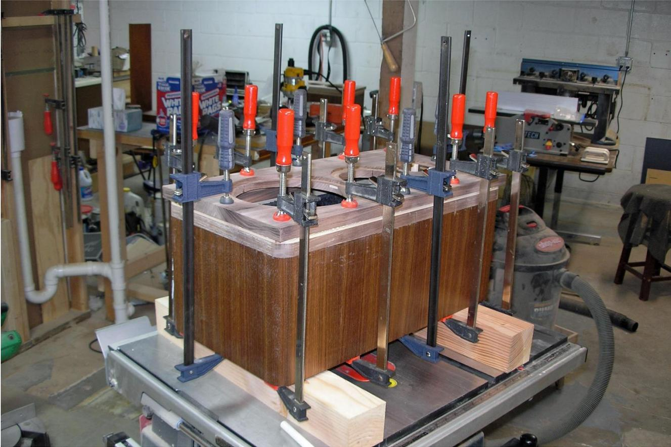
Cutting 1 1/2" bevel on front baffle.
