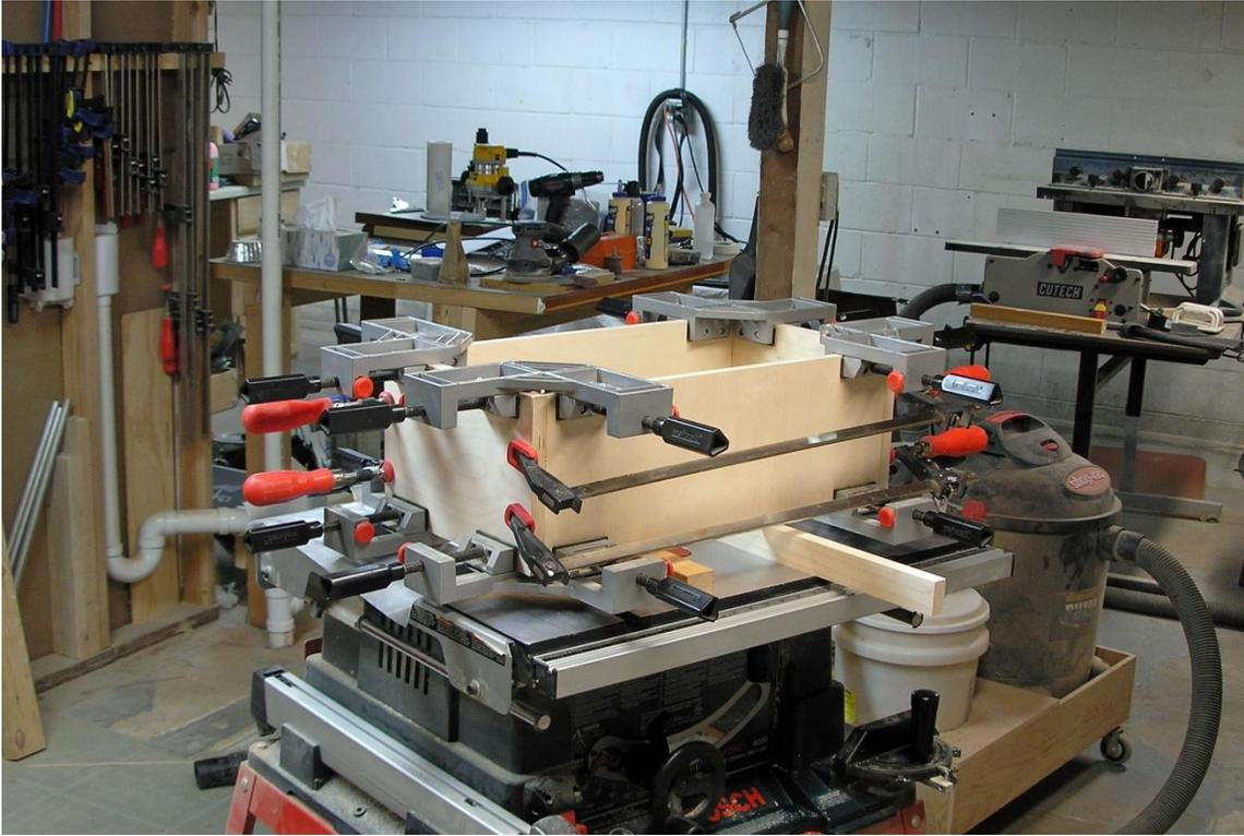
Adding 1/4" firring strips to 1/2" thick side walls.
